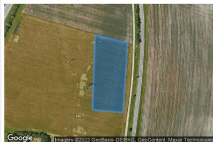
**Name:** PV Feld 4**Footprint area:** 1,606 m<sup>2</sup>**Axis tracking:** Fixed (no rotation)**Tilt:** 20.0 deg**Orientation:** 186.0 deg**Rated power:** -**Panel material:** Smooth glass with AR coating**Vary reflectivity with sun position?** Yes**Correlate slope error with surface type?** Yes**Slope error:** 8.43 mrad
